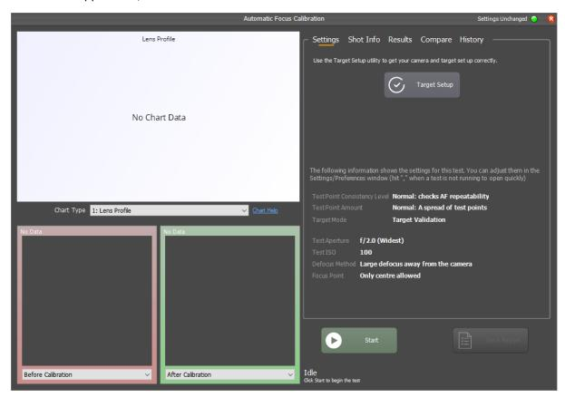
It is important to ensure the environment is correctly set up for a calibration by using the Target Setup utility. You should run the Target Setup utility before running tests or calibrations after any major change - for example moving the camera or target, changing lens, lighting changes etc. The Target Setup utility will confirm for you that everything is ready for the test.
