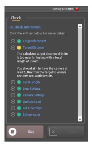
If you need to make any changes to the camera, tripod, lighting etc then do this and click the *Recheck Information* option at the top of the *Check* panel to confirm everything is OK.
